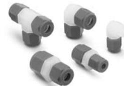
Swagelok PFA tube fittings in sizes from 1/8 to 1/2 in. are available for use with PFA tubing. For more information on Swagelok PFA tube fittings, see the Swagelok *PFA Tube Fittings* catalog, MS-01-05.
